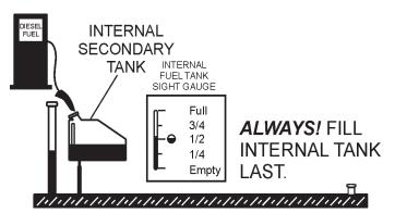
Figure 36. Filling Secondary Internal Fuel Tank
